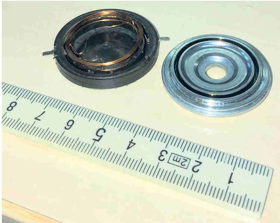
Figure 1.2: Thermal failure of a speaker with 1-inch voice coil. Copper-colored voice coil on the left is mangled.
