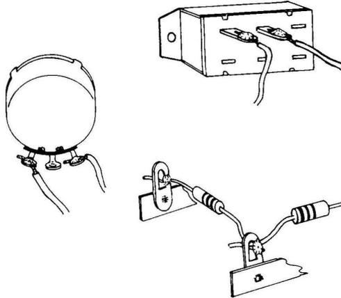
wet the wire is sufficient. Apply a small amount of solder to the place where the wire is to be connected (sometimes, solder from a previous connection will work here). Now hold the wire and the tip of the soldering iron against the terminal until solder flows between the two. Hold the wire so that it does not move until the joint cools, and the connection is complete.
