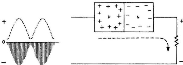
ON THIS HALF OF THE INPUT SIGNAL ..... NO ELECTRON CURRENT CAN FLOW THIS WAY
