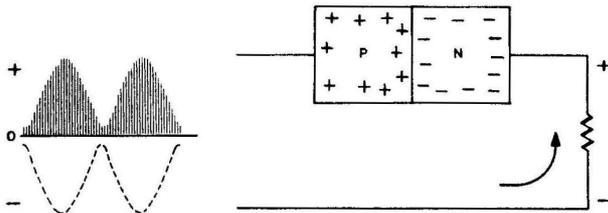
ON THIS HALF OF THE INPUT SIGNAL ..... ELECTRON CURRENT FLOWS THIS WAY
