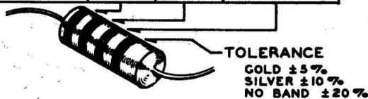
The physical size of a composition resistor is related to its wattage rating. Size increases progressively as the wattage rating is increased. The diameters of 1/2 watt, 1 watt and 2 watt resistors are approximately 1/8", 1/4" and 5/16", respectively.
