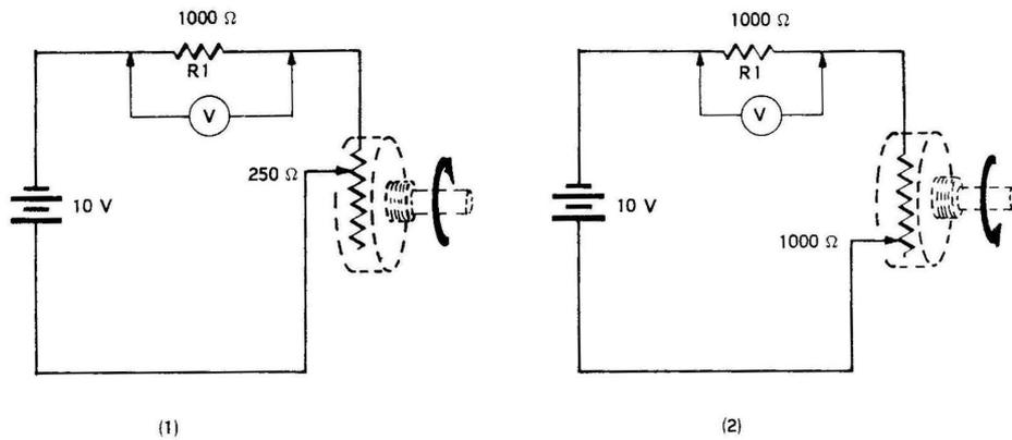
$$\text{CIRCUIT CURRENT} = \frac{\text{TOTAL } E}{\text{TOTAL } R} = \frac{10}{1250} = 8 \text{ MA.}$$
