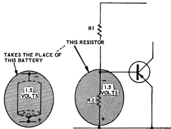
The signal current from the potentiometer is connected across resistor R2 by means of the capacitor, this causes the audio signal currents to flow through resistor R2. These small signal currents also flow from the Emitter to the Base of the transistor just as the small DC currents did in previous lessons.
