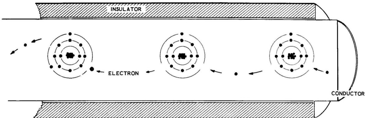
A GREATLY ENLARGED VIEW OF THE ELECTRONS FLOWING FROM ATOM TO ATOM IN A LENGTH OF WIRE
