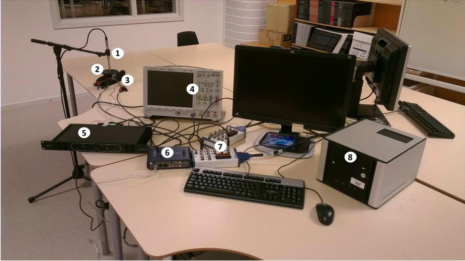
**Figure 6.1:** Laboratory equipment overview. 1. Microphone, 2. Loudspeaker, 3. Stabilising woollen hat, 4. Oscilloscope, 5. AC amplifier, 6. Sound card, 7. Measurement devices, 8. xPC target computer.
